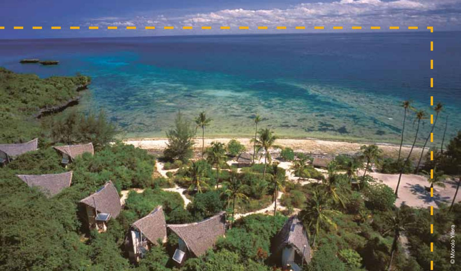
from Zanzibar Island and brought across by sailing dhow on a high tide to avoid damage to the coral reef. Casuarina poles were used for the main structural components, formed into shell-like roof shapes to facilitate rainwater collection and covered with palm thatch (*makuti*).
