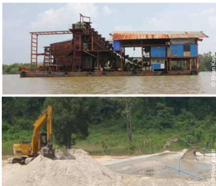
Figure 11: Photograph of sand mining vessel (top) and mining operations (bottom) 3 km south and 0.5 km south of Tatai commune, respectively.
