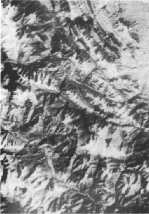
Fig. 4 Simulated false-color infrared image of Scene 1 as displayed on color additive viewer. Growing vegetation appears in shades of red in viewer and shades of grey in this photo.
