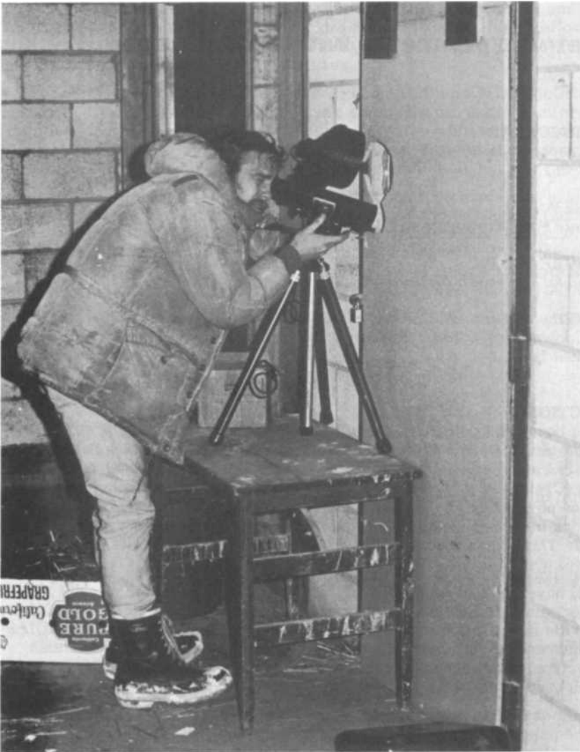
Fig. 1 An infrared scope (shown here without the light-blocking drape) was used to observe the hibernating bear (Fig. 1A) without disturbing him.
