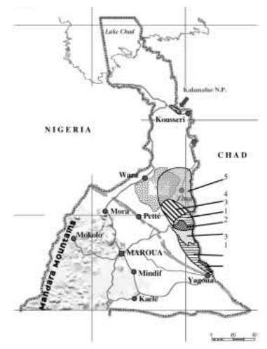
Figure 3.4 After the construction of the dam at Maga, the natural flooding region was expected to be replaced by: 1) irrigated schemes, approx. 12,000 ha, 2) a reservoir, Lake Maga, approx. 39,000 ha, 3) an adjacent zone where flooding no longer would occur, approx. 59,000 ha, 4) a zone in which natural flooding would significantly have changed approx. 50,000 ha, and 5) a zone in which natural flooding would only slightly be affected, approx. 50,000 ha. After Drijver and Marchand (1985).
