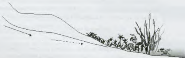
Fig. 1.9(b) Groundwater spring or seep wetland (after Mitsch & Gosselink 1993)
