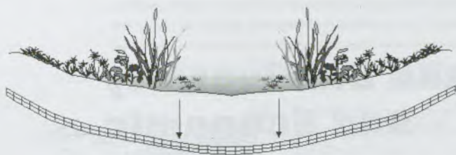
Fig. 1.9 (e) Surface water depression wetland (after Mitsch & Gosselink 1993)
