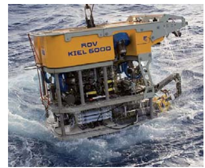
ROV KIEL 6000 (IFM-GEOMAR) has been designed for scientific purposes with an operational depth rating of 6000 m
