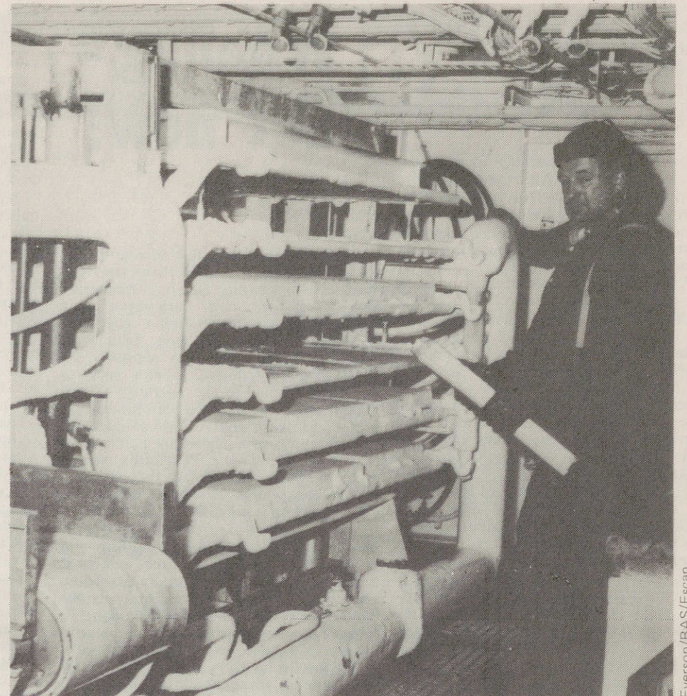
Krill is frozen into solid blocks aboard a West German fisheries research ship for transport from the Antarctic to Europe.
