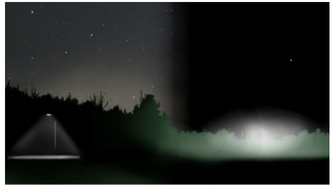
Figure 1.7. Shielded and unshielded lights, glare and the night sky. Source: Robert Dick
