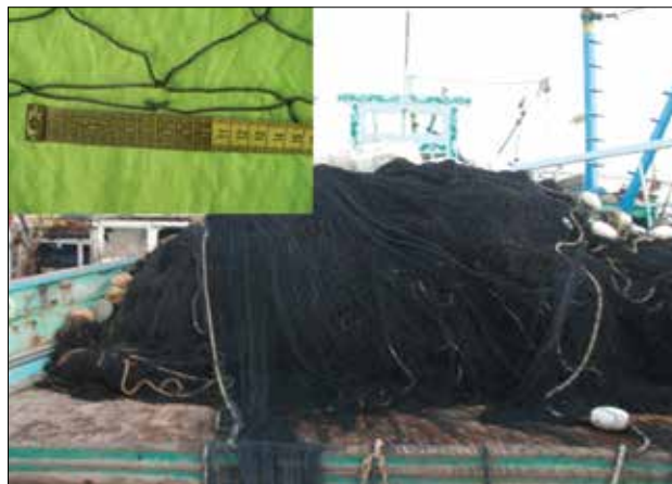
Fig. 3. Polyamide gillnet stored on board tuna fishing vessel at Karachi. Inset: stretched mesh.
