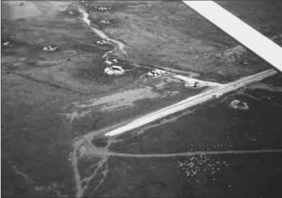
*Photo 2.1 The dyke along the Logone, completed in September 1982, prevented water to enter the floodplain through the Petit Goroma (Photo Piet Wit).*
