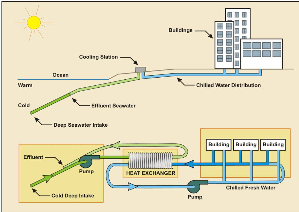
Fig. 1. Schematic diagram of a SWAC system
