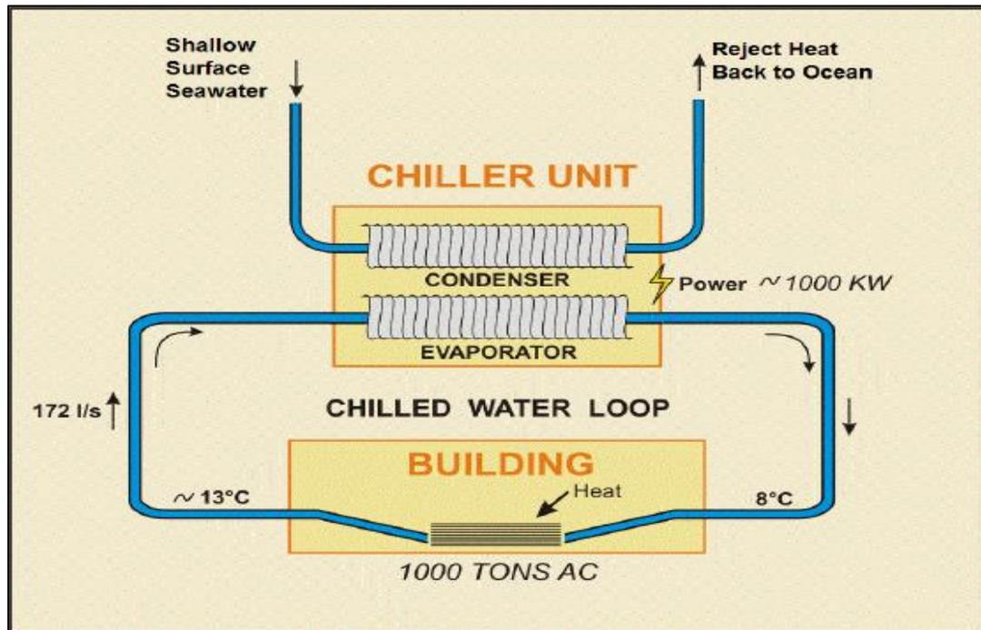
Fig. 2. Schematic diagram of a seawater cooled conventional air conditioning condenser.
